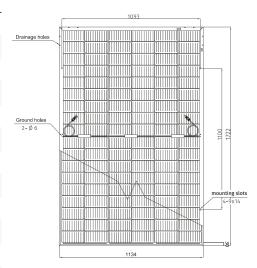
Note: dimensions in mm, tolerance +/- 2 mm
